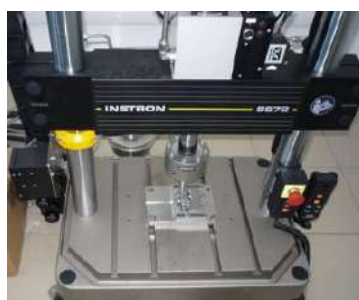
Dental implants fatigue testing
